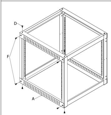
Attach the other Front/Back Frame (A) to the frame built above and secure them with 4 of the M6\*12mm Screws (D), 4 of the M6 Flat Head Screws (F) and 8 of the M6 Flange Nuts (E) using a Phillips Screwdriver.
