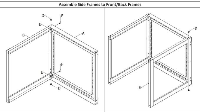
Attach Side Frames (B) to one of the Front/Back Frames (A) and secure them with 4 of the M6\*12mm Screws (D), 4 of the M6 Flat Head Screws (F) and 8 of the M6 Flange Nuts (E) using a Phillips Screwdriver.
