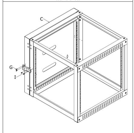
Attach Latch (I) to the Frame built above (on the opposite side of the frame in which you installed the Hinges (H)and secure them with 4 of the M4 Tapping Screws (G) using a Phillips Screwdriver.
