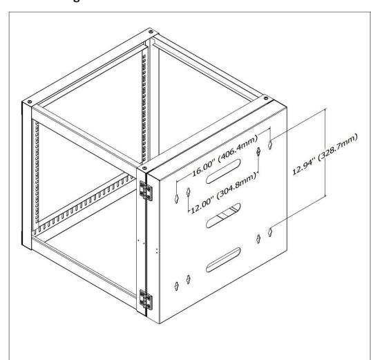
Attach the rack to a wall or other suitable mounting surface using appropriate anchors. (The included Anchors (J) are intended to be used on a concrete wall.)
