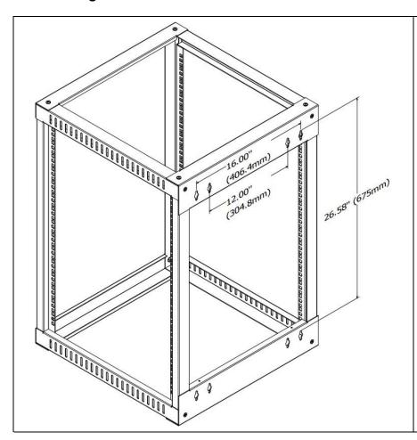
Attach the enclosure to a wall or other suitable mounting surface using appropriate anchors. The included Anchors (G) are intended for use on a concrete wall.
