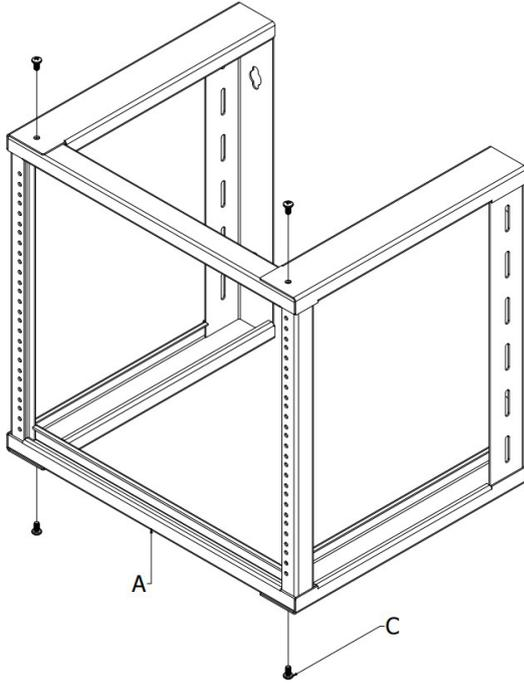
Attach Front Frame (A) to the Side Frames (B) and secure them with 4 of the M6 Screws (C) using a Phillips Screwdriver (not included).
