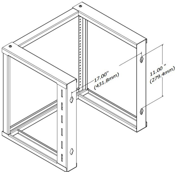
Attach the rack to a wall or other suitable mounting surface using appropriate anchors. The mounting holes are spaced 17" (431.8mm) as reflected in the diagram.
