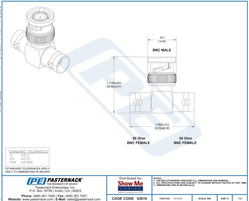
BNC Tee Adapter Female-Male-Female PE9001 CAD Drawing
