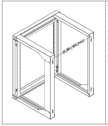
Attach the rack to a wall or other suitable mounting surface using M6 Wall Mounting Screws (L) and M6 Metal Washers (K). Mounting holes are spaced 18.28" (464.2mm) as reflected in the diagram.
