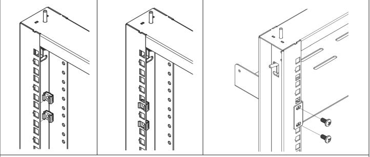
**1** Locate the numbered square openings in the Equipment Mounting Frame (C) where you plan to install your equipment. Install M6 Cage Nuts (I) into the square openings to provide an attachment point for the M6 Mounting Screws (H). Note: Consult your equipment documentation to determine how many cage nuts will be required and where they will need to be installed.
