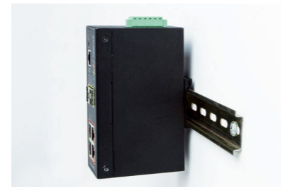
Figure 5-2: Complete DIN-rail mounting
