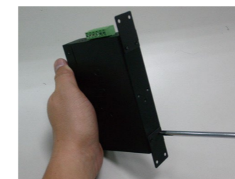
Figure 5-4: Placing Wall-mount Plate on Industrial Device
