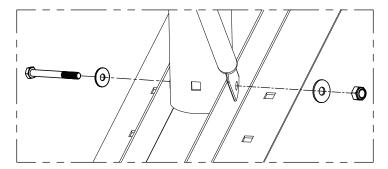
Before assembly supporting rod, release screw and nut, then use same screw, washer, nut fixed supporting rod and mast pole on the base mount
