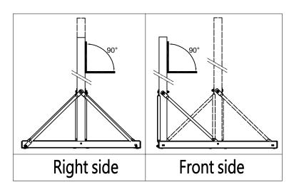
Adjust pole angel to 90 degree then tighten all screw
