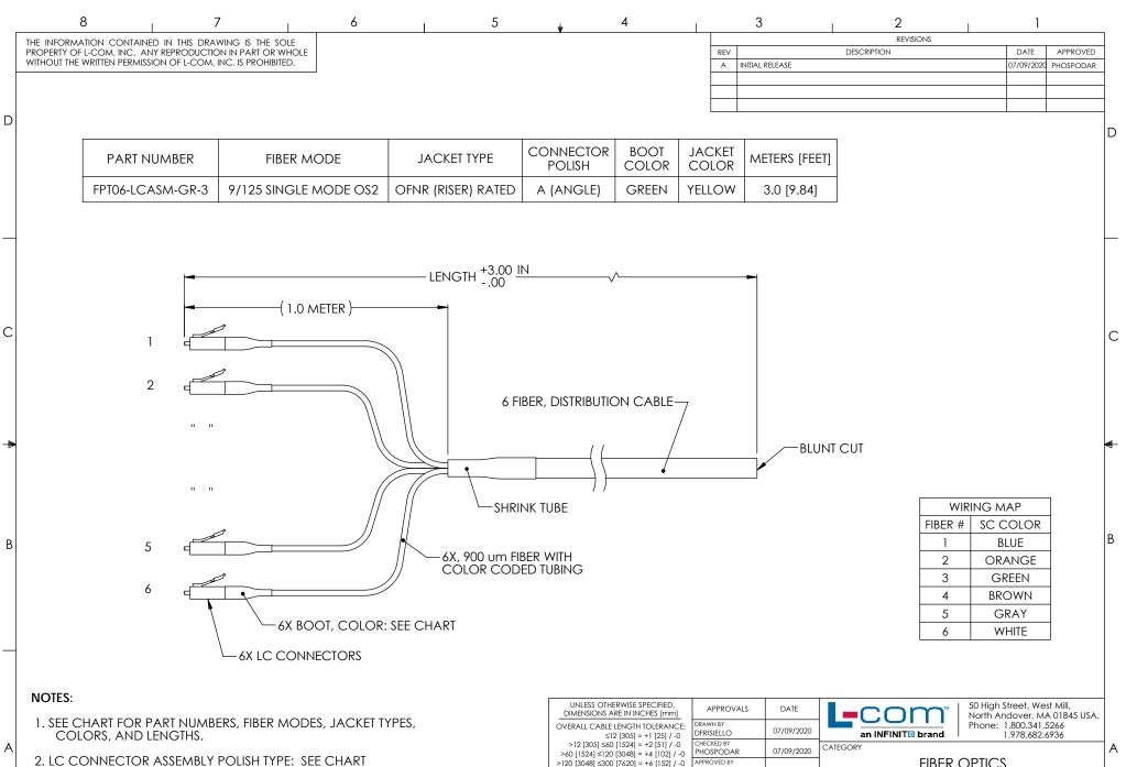
3. ALL CONNECTORS ACCOMPANIED WITH A DUST CAP INSTALLED (NOT SHOWN).
