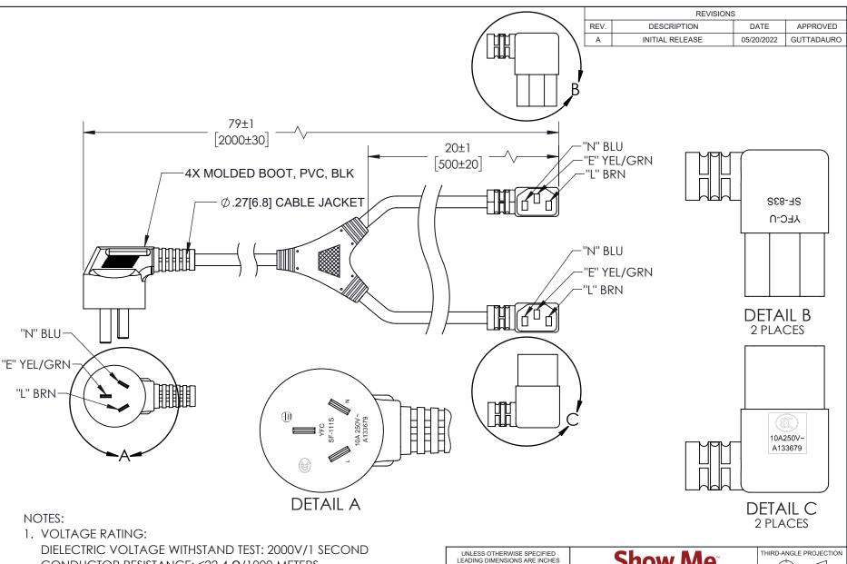
CONDUCTOR RESISTANCE: ≤22.4 \(\Omega/1000\) METERS **VOLTAGE RATING: AC 300/500V**
