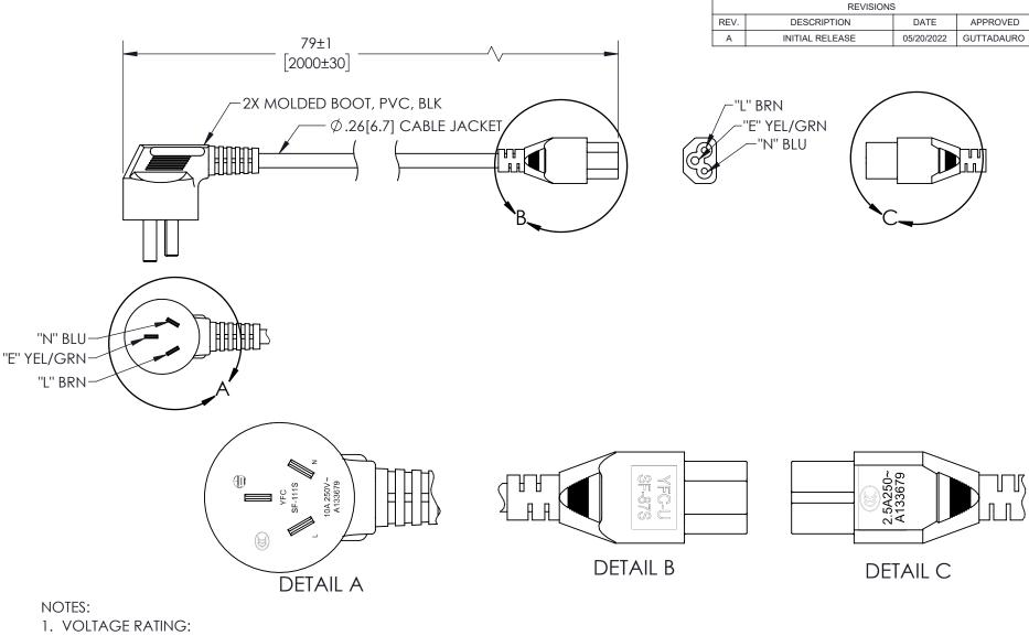
DIELECTRIC VOLTAGE WITHSTAND TEST: 2000V/1 SECOND CONDUCTOR RESISTANCE: ≤22.4 \(\Omega/\)1000 METERS **VOLTAGE RATING: AC 300/500V**
