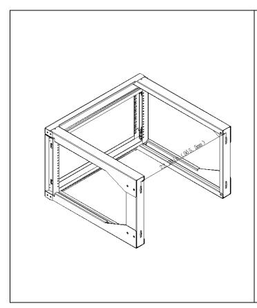
Attach the rack to a wall or other suitable mounting surface using M6 Wall Mounting Screws (L) and M6 Metal Washers (K). Mounting holes are spaced 22.26" (565.5mm) as reflected in the diagram.
